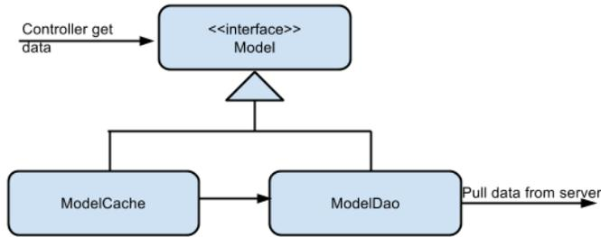
Figure 6: Proxy Cache Structure
