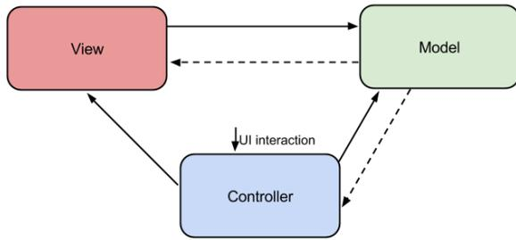
**Figure2: MVC Structure**
