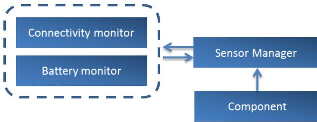
**Figure 11 : Sensor Manager Structure**
